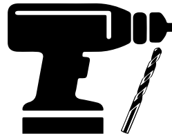
Drill and drill bits Perceuse et forets Taladro con brocas ø1/8" (3mm) & ø3/16" (4mm) & ø5/16" (8mm)
